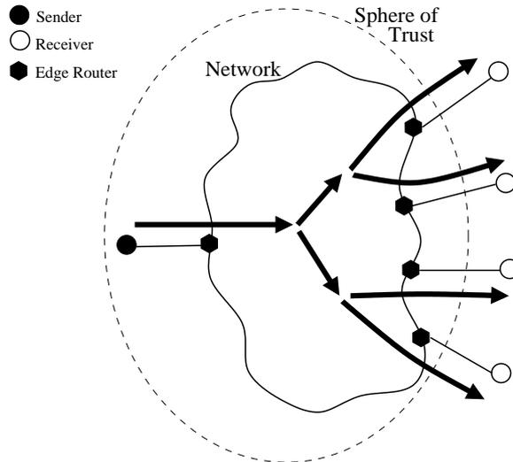
Figure 2.1: Multicast congestion control with distrusted receivers
