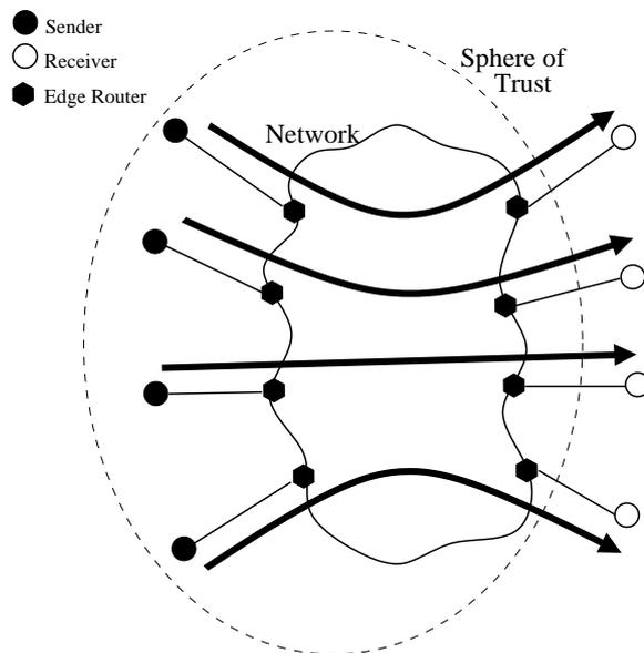
Figure 2.2: Unicast congestion control with distrusted receivers
