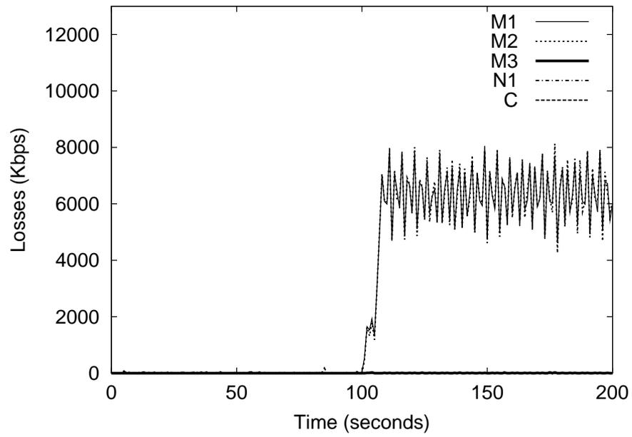
Figure 2.7: Manipulation with feedback suppression in pgmcc
