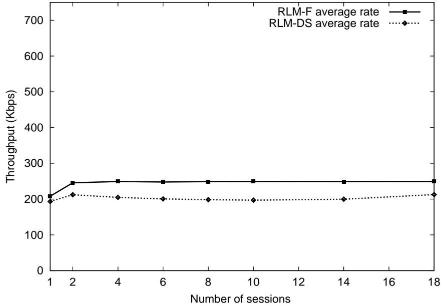
Figure 4.12: Average throughput in RLM-F and RLM-DS
